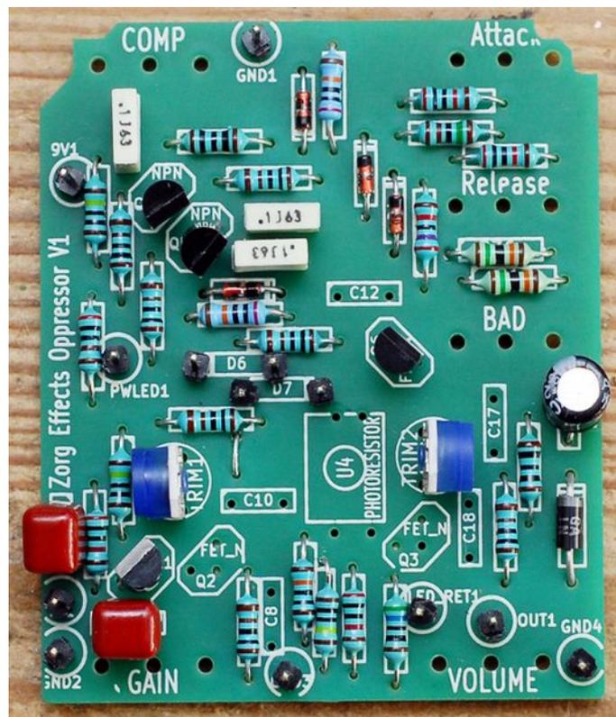
Add the optocoupler. Be careful of its direction (See below), the "led+" text must be on top with the "+" on the left.
