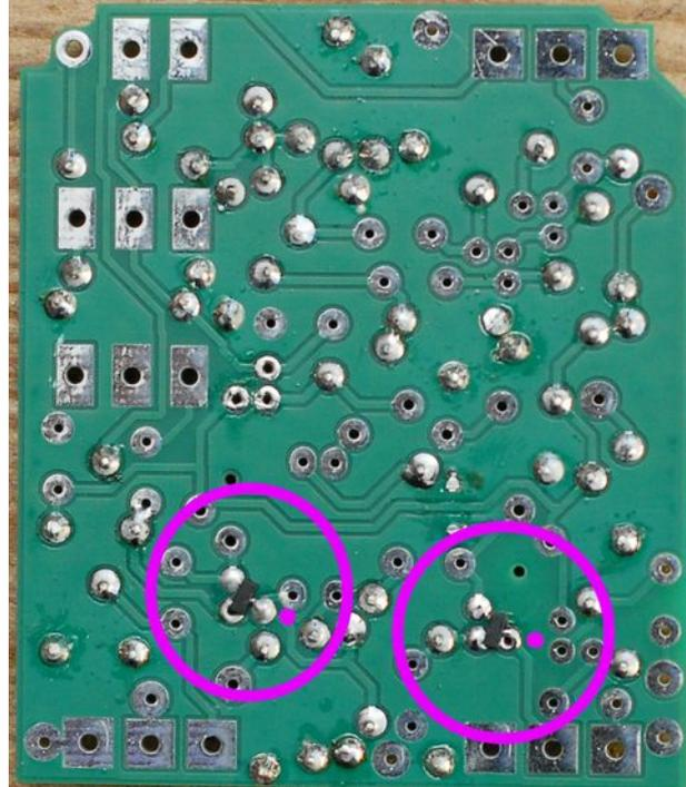
Flip the board and solder the jumper by using resistance's legs.
