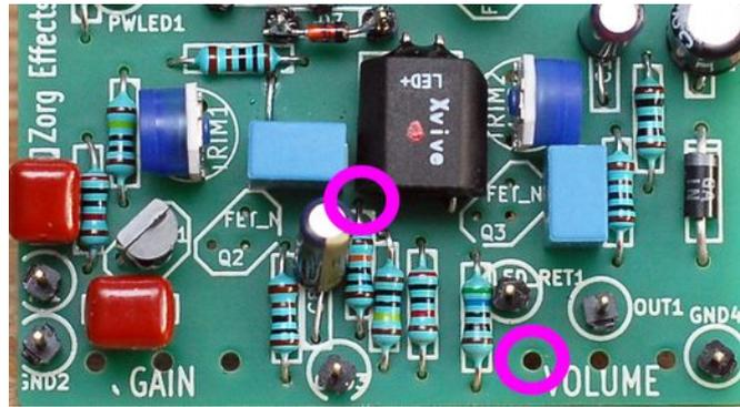
Then set the gain pot a bit upper than the minimum and do the same for the volume pot test point (see picture above). Then for each stage, level the gain or your input signal so that you can work with a very slightly saturated signal and trim the pots for the best gain.
