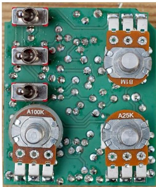
Then just after soldering, you must test that your switch's solders are ok. **This stage is really important: 99% of your problems will come from a badly soldered switch!!!**
