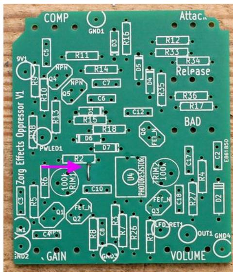
Then we're going to solder components from the smaller to the taller. First, diodes and resistances. You shall take care of the diode position. It MUST be on the same direction as on this picture :
