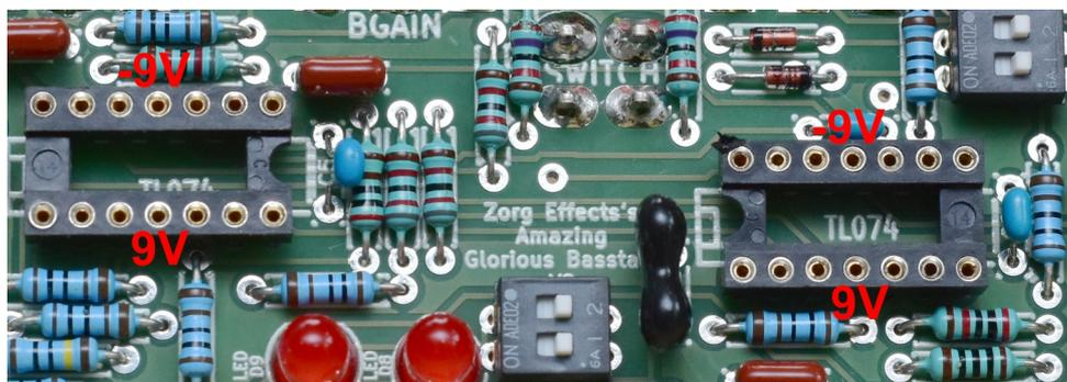
Step 4: insert the TL074 in socket U2 and the TLE2074 in socket U3.
