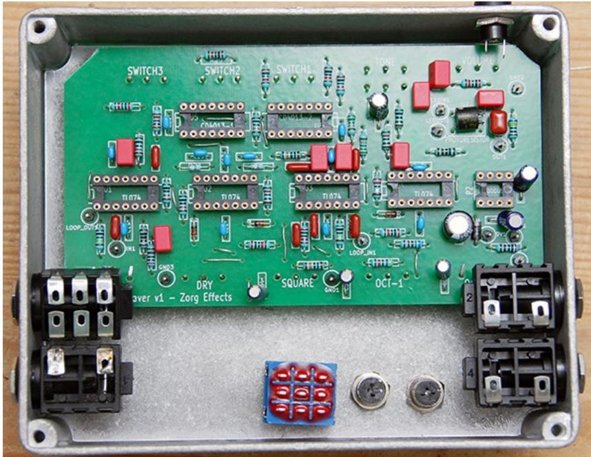
Now you can screw the audio jacks, led socket, footswitches and DC jack. The loop jack might be a little leaning because of the board under it. Take care that the jacks legs do not touch components on the board. The stereo jack must be put at the position like the picture above.
