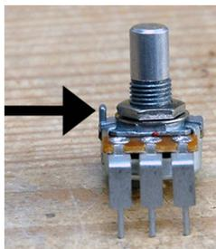
Stick 16mm length of window insulator under each pot. It's in order to prevent solders on the board to connect with the body of the pot and shortcut some circuits.
