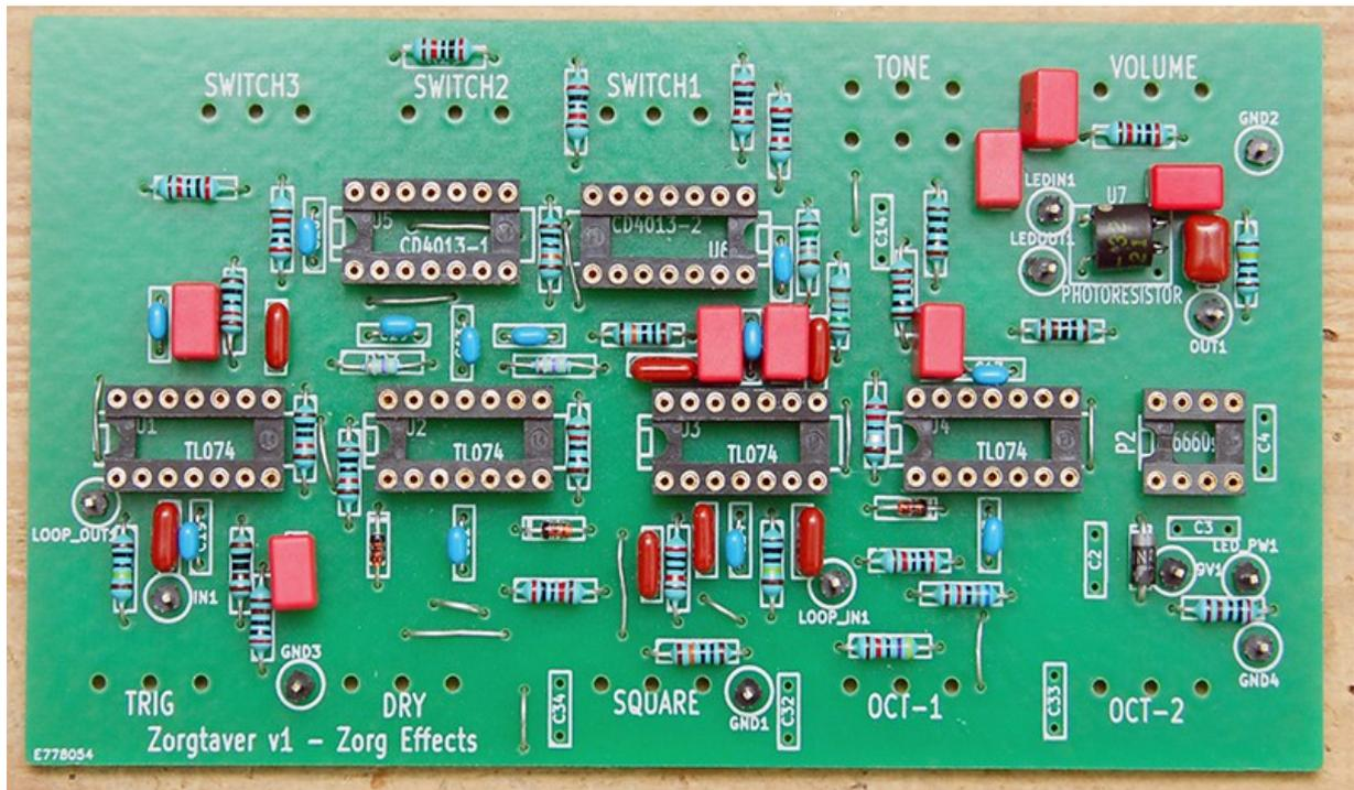
Check out the direction for the NSL-32, the white dot must be left side on top :
