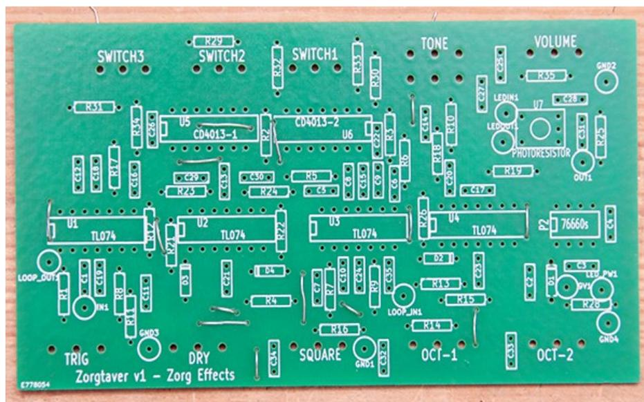
Then we're going to solder components from the smaller to the taller. First, diodes and resistances. You shall take care of the diodes positions. They MUST be on the same direction as on this picture :
