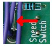
Add the NSL-32. Be careful for the directions too. The white dot must be placed left side and down. Do not fold the LED lugs of the NSL (short ones).
