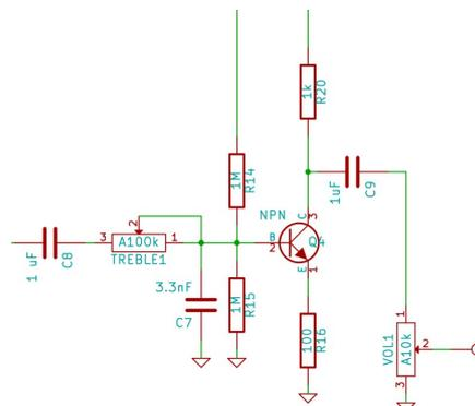
C8 is a decoupling cap, together with R15 it makes a high pass filter, cutting at  $F=1/(2 \times \pi \times C8 \times R15)=15\text{Hz}$ .
